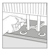
Drill holes two times larger than the diameter of the pipes. Remove a piece of the strip with a utility knife or a saw. Put the strip on one side of the pipes and the removed piece on the other side.
