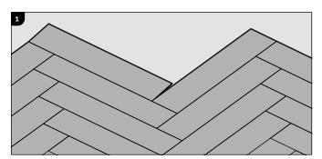
The boards need to be locked into one another, using the 5Gi system. To connect a new board you have to use a rubber hammer.
