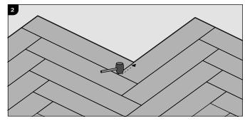
Use a rubber hammer and slightly knock at the 5Gi system to connect the short side. Start in the corner and work towards the end of the board.
