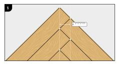
Measure the distance between the two straight lines, originating from the corners of the strips.
